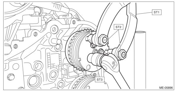
4) Remove the intake cam sprocket LH.
