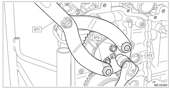
4) Remove the intake cam sprocket RH.
