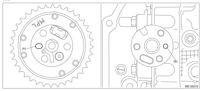
2) Hold the intake cam sprocket RH using the ST1 and ST2, and install the bolts using the ST3.
