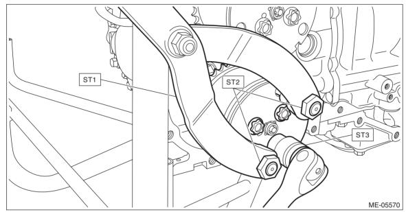
4) Remove the exhaust cam sprocket RH.
