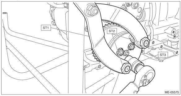
3) Install the timing chain RH. <Ref. to ME(H4DO(w/o HEV))-184, TIMING CHAIN RH, INSTALLATION, Timing Chain Assembly.>
