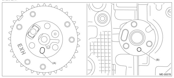
2) Hold the exhaust cam sprocket LH using the ST1 and ST2, and install the bolts using the ST3.
