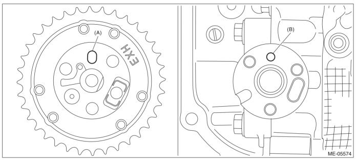
2) Hold the exhaust cam sprocket RH using ST1 and ST2, and install the bolts using ST3.
