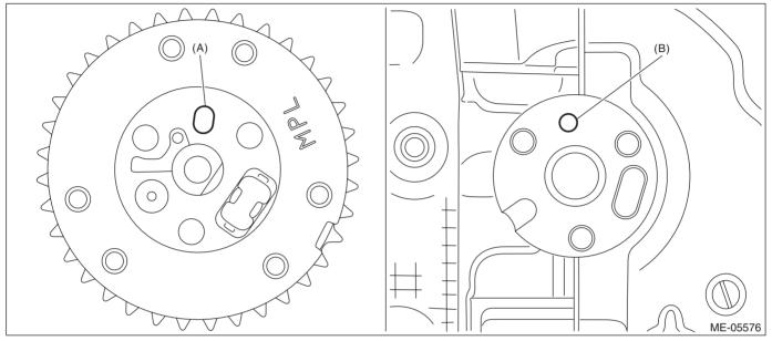
2) Hold the intake cam sprocket LH using the ST1 and ST2, and install the bolts using the ST3.
